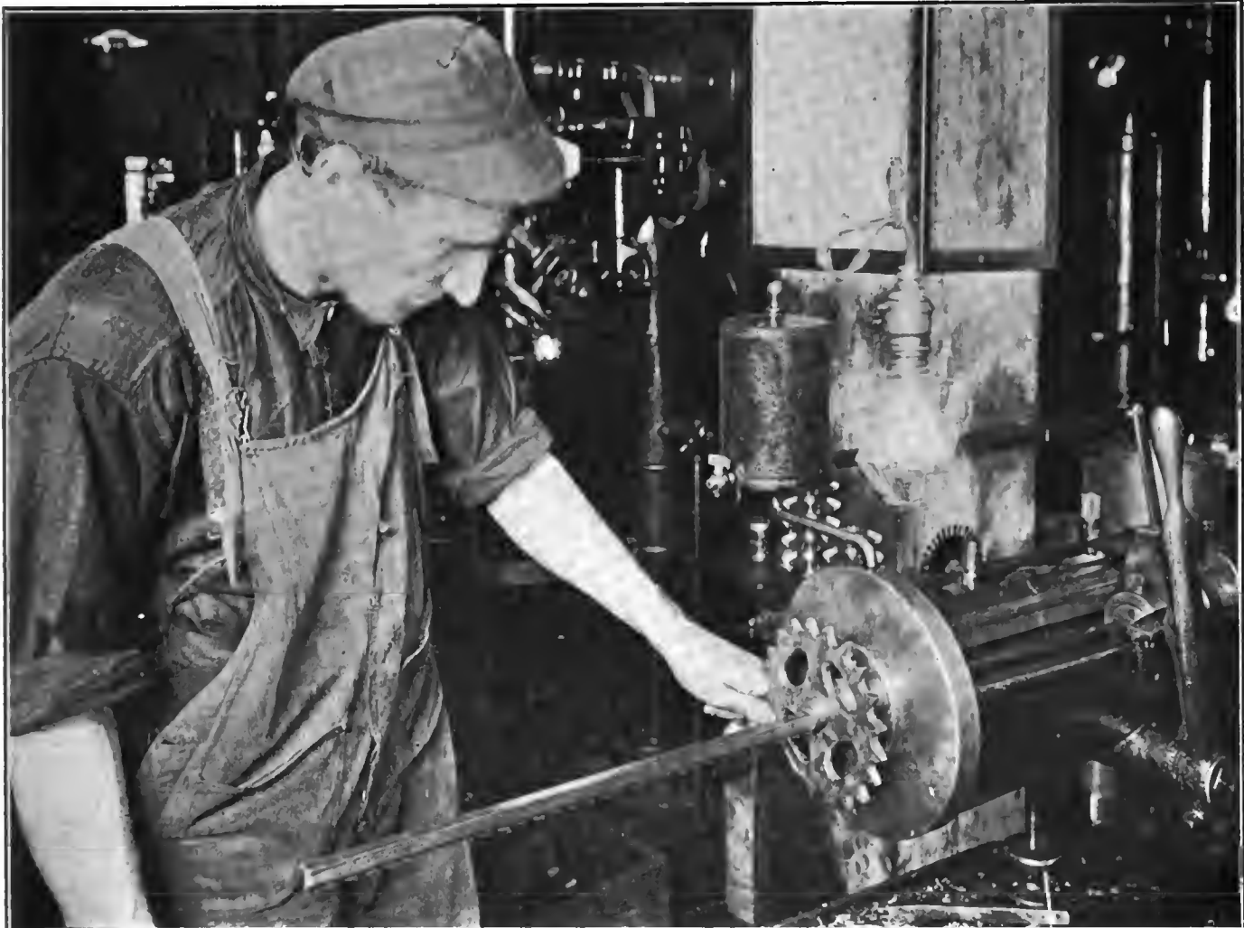
ILLUSTRATING METHOD EMPLOYED IN BROACHING SQUARE HOLES IN SPROCKET WHEELS AND GEARS AT WOODS PLANT
